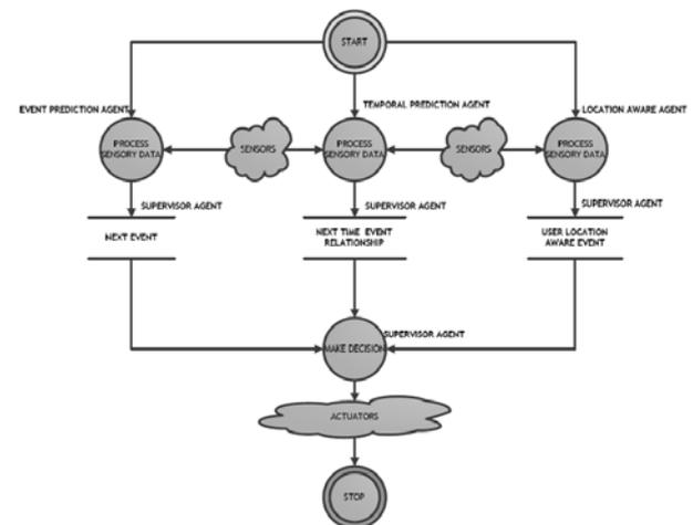
Figure 4. Activity diagram of the proposed multiagent system
