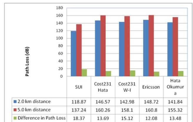
**Figure 2.** A comparison of results for urban area at 6 m receiver antenna height and 2.5 GHz
