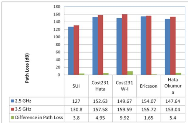
**Figure 3.** A comparison results for urban environment at 3 km distance and 6 m of receiver antenna height
