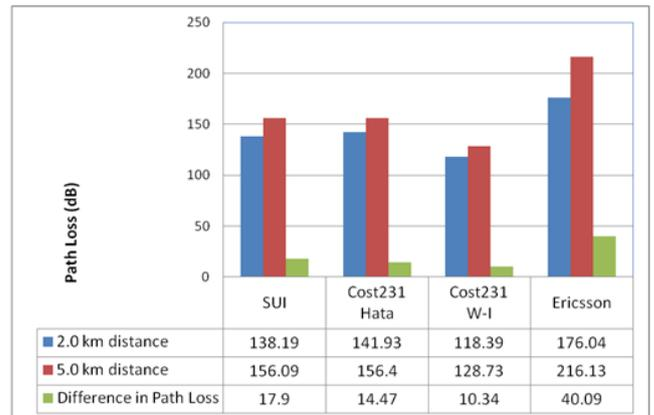
**Figure 8** A comparison of simulation results for rural area at 6 m receiver antenna height and 2.5 GHz
