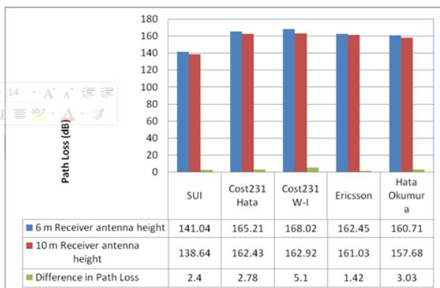
**Figure 4.** A comparison of results for urban environment in at distance of 5 km and 3.5 GHz operating frequency
