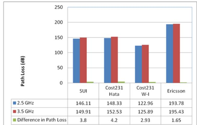
**Figure 9** A comparison of results for rural area at distance of 3 km and 6m of receiver antenna height.
