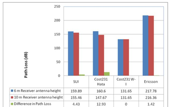
**Figure 10** A comparison of simulation results for rural environment at 5 km distance and 3.5 GHz
