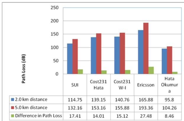
**Figure 5.** A comparison of simulation results for suburban area at 6 m receiver antenna height and 2.5 GHz
