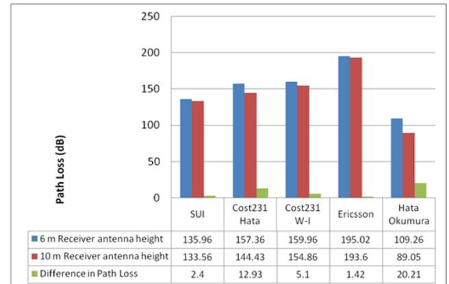
**Figure 7.** A comparison of simulation results for suburban environment at 5 km distance and 3.5 GHz
