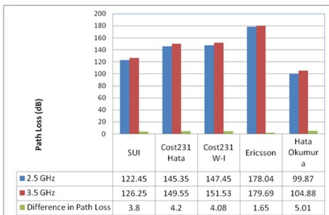
**Figure 6.** A comparison of results for suburban area at distance of 3 km and 6m of receiver antenna height.
