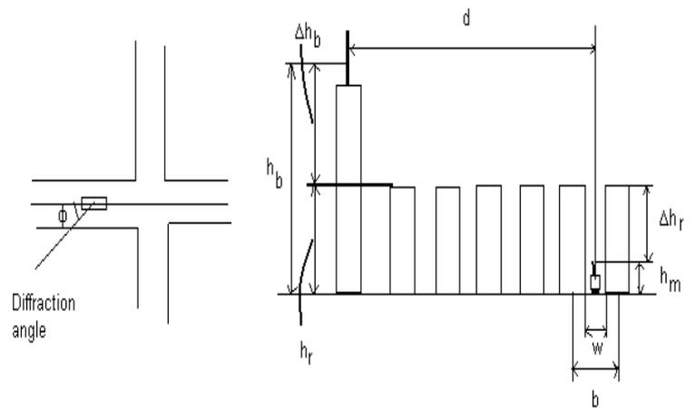
Figure 1. Diffraction angle and urban scenario
