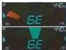
Fig. 13. Universal tuner display (upper photo when frequency is too low; lower photo when frequency is appropriate)
