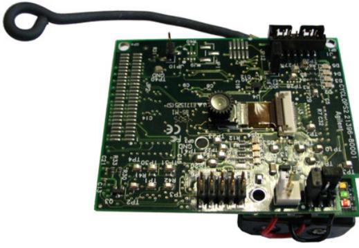
Fig. 1. A camera node consisting on a Cyclops camera attached to a Mica2 mote.
