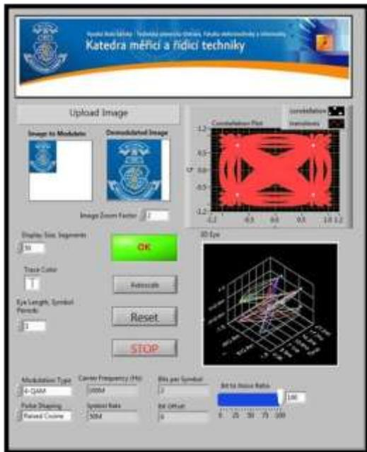
**Figure 9.** Front-panel: 4-QAM Screenshot with maximum Bit to Noise Ratio
