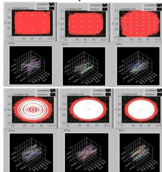
**Figure10.** Constellation and 3D Eye diagram for M-QAM with Bit to Noise Ratio (100) respectively for (8, 16, 32, 64, 128 and 256)
