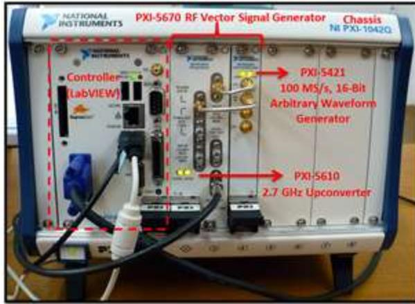
**Figure 3.** Vector Signal Generator (NI PXI-5610 – RF Upconverter, NI PXI-5421 -100MS/s AWG)
