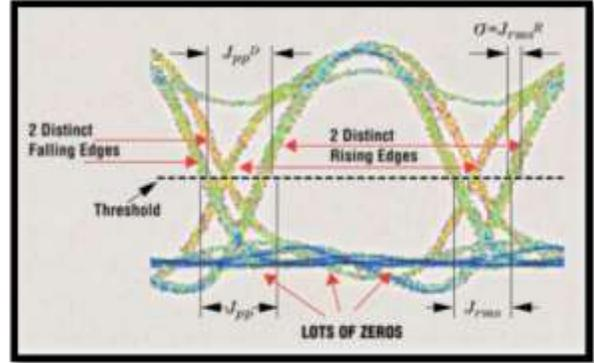
**Figure 6.** An eye diagram with an irregular shape provides a wealth of information
