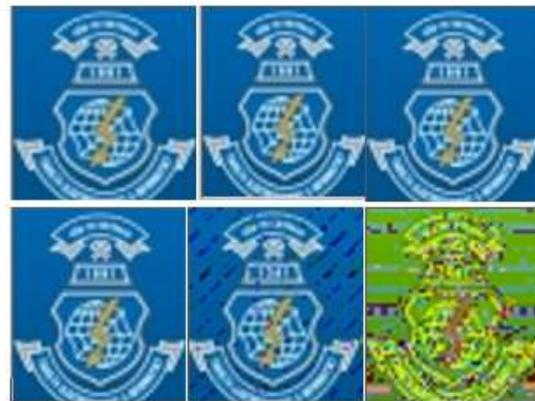
**Figure12.** Demodulated Image with Bit to Noise Ratio 100 respectively for M-ary QAM (8, 16, 32, 64, 128 and 256)
