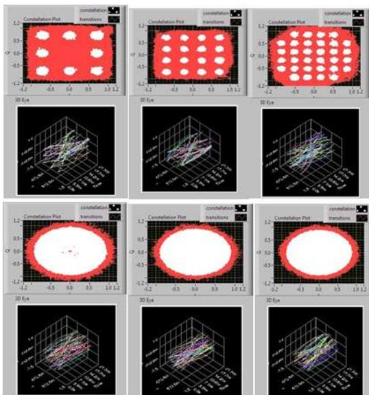
**Figure11.** Constellation and 3D Eye diagram for M-QAM with Bit to Noise Ratio (30) respectively for (8, 16, 32, 64, 128 and 256)
