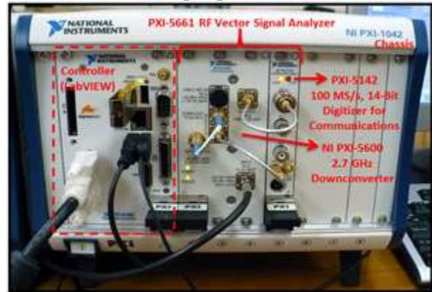
**Figure 4.** Vector Signal Analyzer (NI PXI-5600 – RF Downconverter, NI PXI-5142 - 100MS/s OSP Digitizer)
