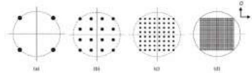
**Figure 2.** Square QAM constellations: a) 4-QAM (QPSK), b) 16-QAM, c) 64-QAM, d) 1024-QAM
