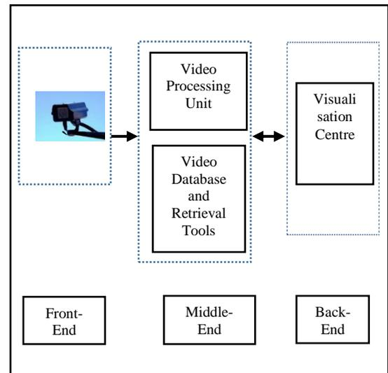
**Figure 1: Architecture of video surveillance system**
