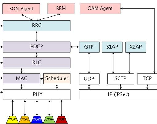
**Figure 3.** LTE Protocol Stack Interaction for Carrier Aggregation
