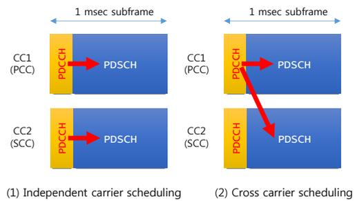
**Figure 4.** Resource Scheduling with Downlink Control Channel Signaling
