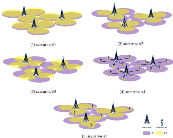
Figure 2. Carrier Aggregation Deployment Scenarios (F2 > F1).
