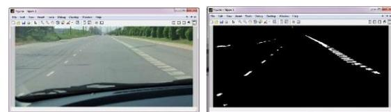
(a) Road part image (b) Extracted line Segment image
