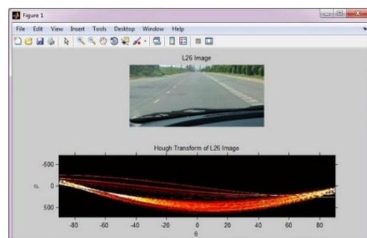
Figure 2. Detecting line road by using the Hough transform
