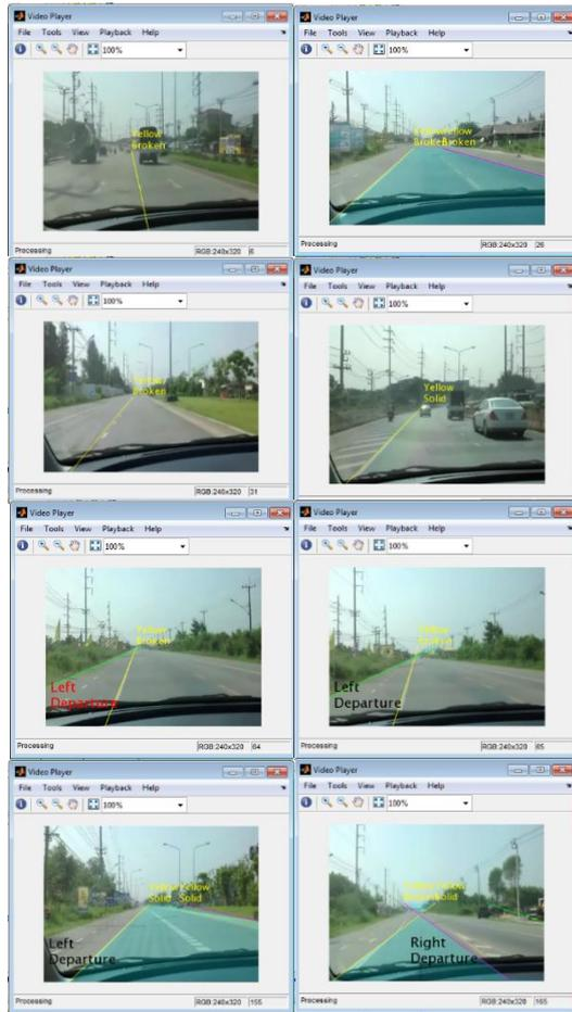
Figure 7. Real-time lane detection for driving system Using Image Processing Based on Edge detection and Hough transform.
