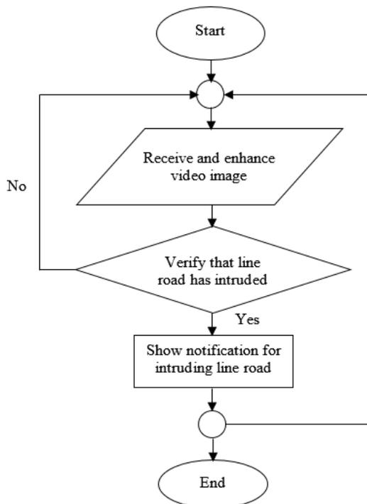
Figure 5. Frame work of Real-time lane detection for driving system Using Image Processing Based on Edge detection and Hough transform.
