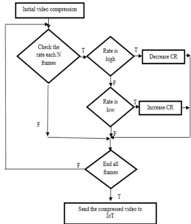
Fig. 4. Flow Chart of the CS video technique based on available bandwidth
