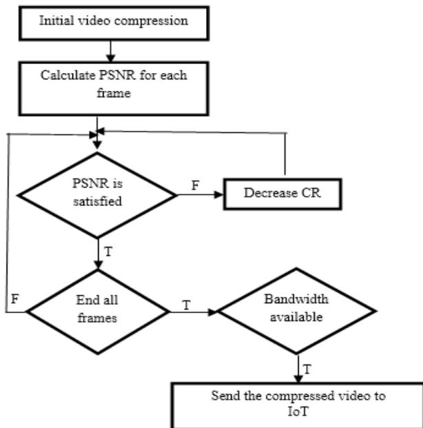
Fig. 3. Flow Chart of the CS video technique based on QC
