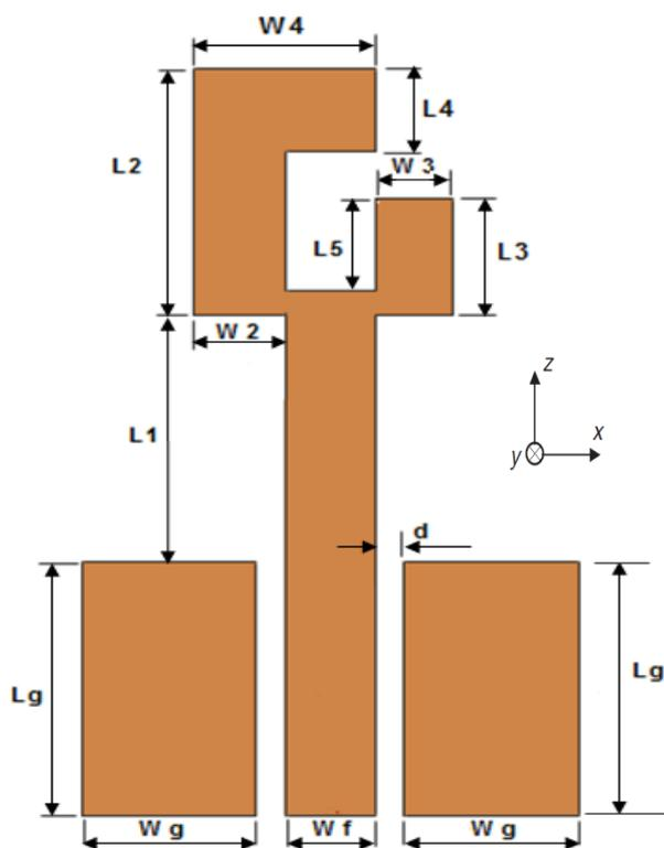
Figure 1. Geometry of the simulated antenna
