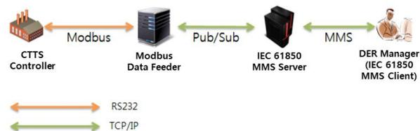
**Figure 1.** Core Components of an IEC 61850 Communication System for DER Management
