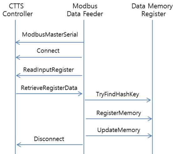
**Figure 3.** Mesasage flow between CTTS Controller and Modbus Data Feeder
