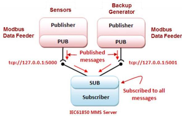
**Figure 2.** ZeroMQ Pub-Sub Pattern Between MMS Server and Modbus Data Feeder
