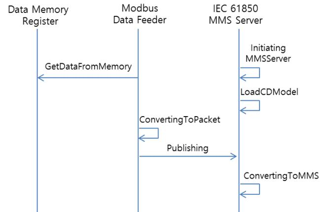
**Figure 4.** Message flow between Modbus Data Feeder and MMS Server
