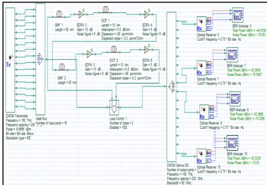
Figure 1. The main layout for the 16x40Gbps DWDM system.
