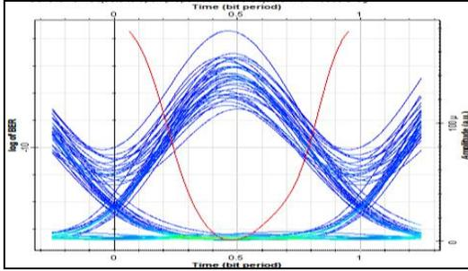
Figure 9. BER analyzer for output channel\_16 (193THz) when span=120km.
