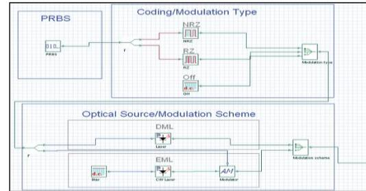
Figure 3. The block diagram for each DWDM channel transmitter.
