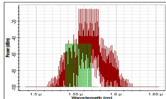
Figure 6. OSA for all channels when span link=100km.
