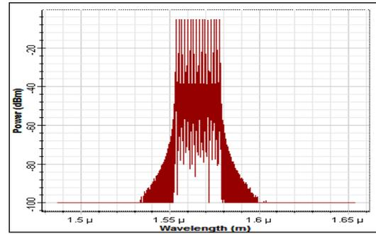
Figure 5. OSA for all 16-channels when span link=0km.
