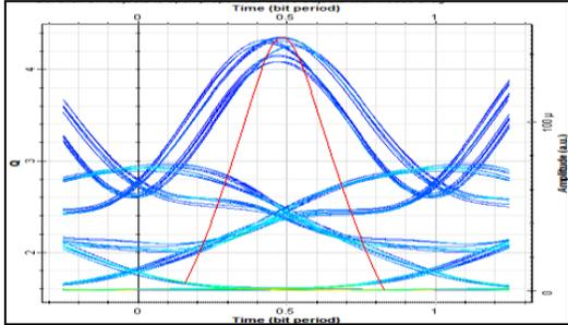
Figure 10. Q-Factor for the output channel\_1 (190THz) when span=120km.
