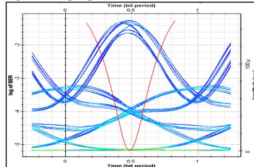
Figure 8. BER analyzer for output channel\_1 (190THz) when span=120km.
