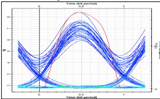
Figure 11. Q-Factor for the output channel\_16 (193THz) when span=120km.
