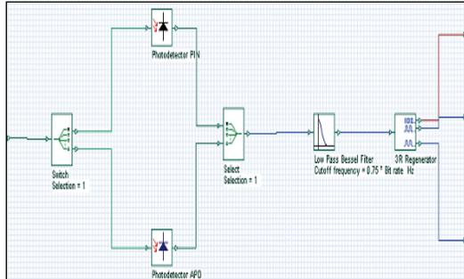
Figure 4. The optical receiver subsystem (Green Lines means optical signal, Blue means electrical signal, and Red means digital signal).
