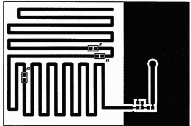
**Figure 3.** The meander antenna under investigation with three minor modified designed points.
