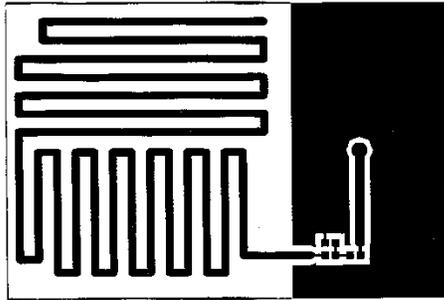
**Figure 1.** Intended meander antenna design under investigation.
