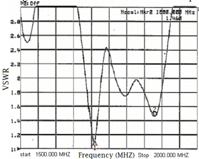
**Figure 6.** VSWR with resistance point number 3, shown in Figure 3, disconnected. At 1710 MHz the SWR = 1.108 and at 1880 MHz the SWR = 1.460.
