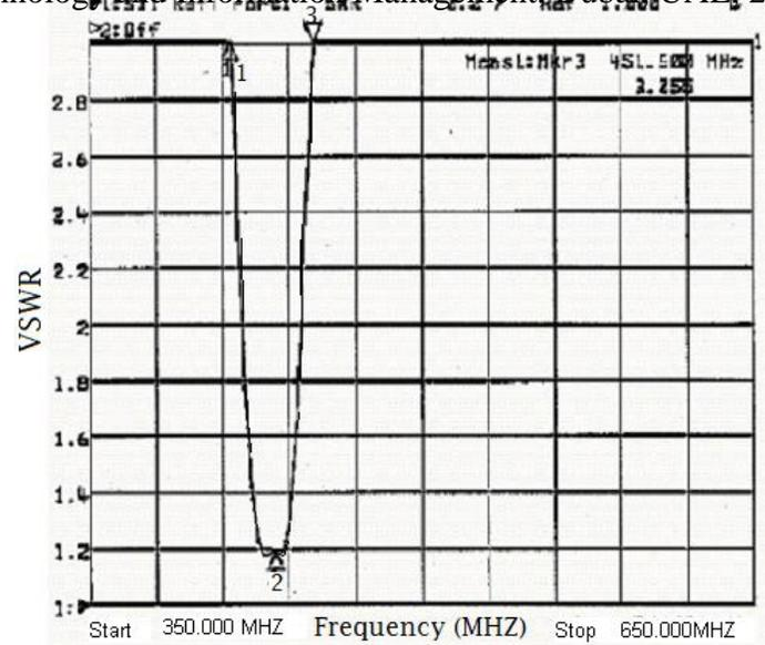
**Figure 5.** VSWR with resistance point number 2, shown in Figure 3, disconnected. At 433.9 MHz the SWR = 1.195.
