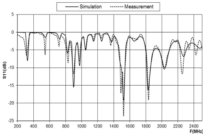
**Figure 2.** Simulation versus measurement results for the constructed meander antenna under investigation in the 200–2800 MHz frequency band. Solid line: simulation; dashed line: measurements.
