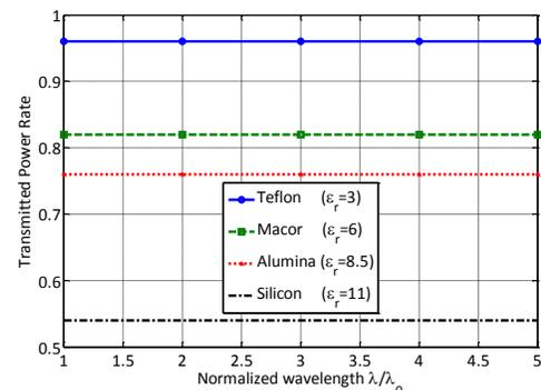
**Figure 1.** Transmitted power rate as a function of normalized wavelength  $\lambda / \lambda_0$  for four different dielectric materials.
