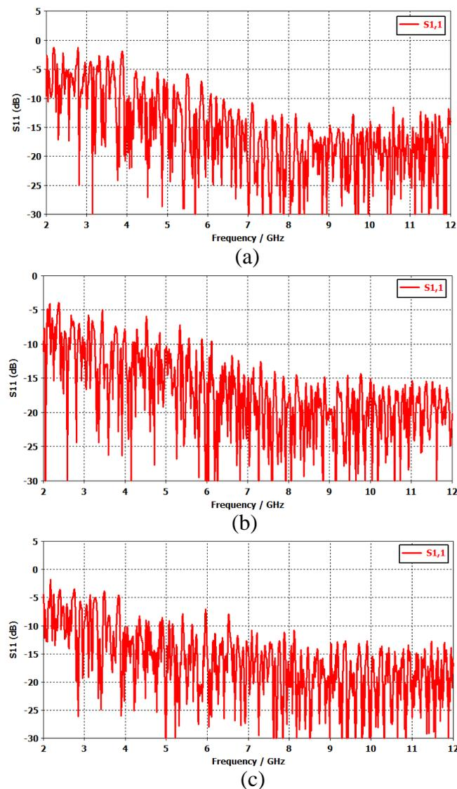
**Figure 5.** Return loss variation of the antennas having (a) 1 ML, (b) 2 MLs and (c) 3 MLs.
