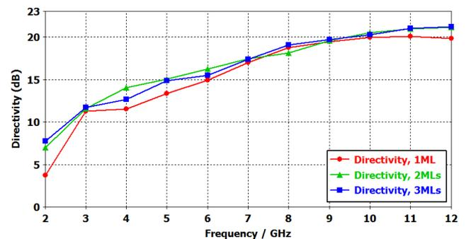
**Figure 6.** Directivity values of dielectric lens antenna having (a) 1 ML, (b) 2 MLs, and (c) 3 MLs.
