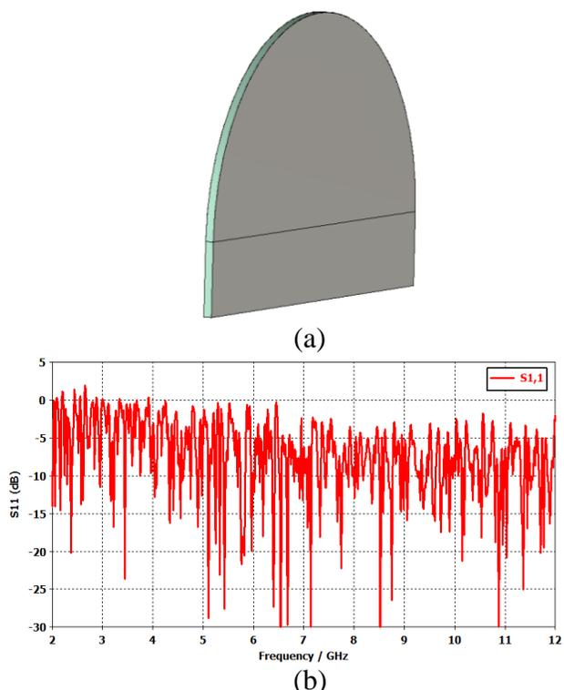
**Figure 3.** The antenna without ML and flaring part (a) geometry, (b) return loss.
