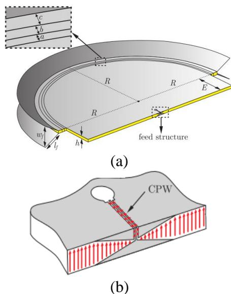
**Figure 2.** Geometry of the (a) antenna and (b) feeding.
