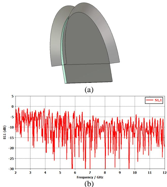
**Figure 4.** The antenna with flaring without MLs (a) geometry, (b) return loss.
