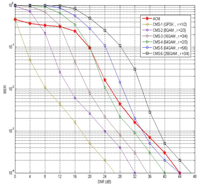
Figure 9. BER performance comparison between BRS cooperative with different CMSs and with ACM,  $N=8$
