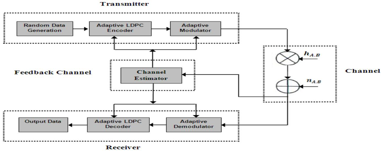
Figure 2. Transceiver structure with adaptive LDPC coded modulation at source node
