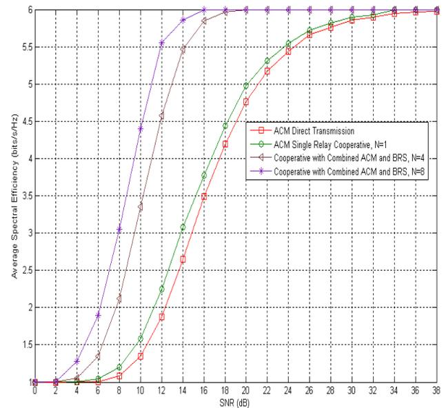
Figure 12. ASE of different transmission scenarios, SNR adaptation threshold at  $BER = 10^{-2}$
