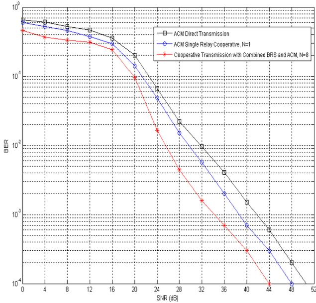
Figure 10. BER performance comparison between ACM direct transmission, ACM cooperative with single relay and Cooperative system with combined BRS and ACM, SNR adaptation threshold at  $BER = 10^{-2}$
