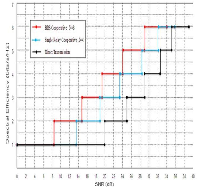
Figure 6. SNR adaptation thresholds of each candidate pair at  $BER=10^{-2}$  for different scenarios of simulations
