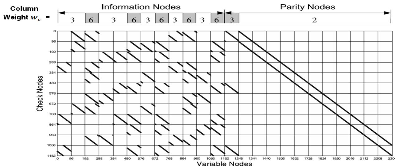
Figure 4. Structure of the parity check matrix  $H$  for a rate  $1/2$  WiMAX 802.16e LDPC code with codeword length  $n=2304$  bit ( $z = 96$ ), where the bold lines represent elements "1" in  $H$
