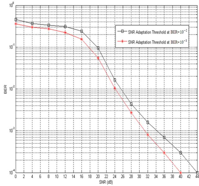
Figure 11. The effect of SNR adaptation threshold on the BER performance of the proposed cooperative system with combined ACM and BRS,  $N=8$
