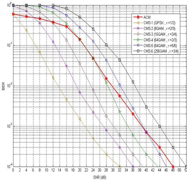
Figure 8. BER performance comparison between single relay cooperative with different CMSs and with ACM,  $N=1$
