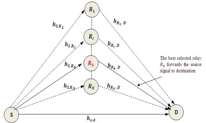
**Figure 1.** Multi-node cooperative communication system with best relay selection
