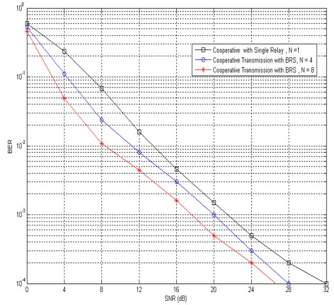
Figure 5. BER versus SNR for different number of relay nodes  $N$ , considering transmission over Rayleigh fading channels ( $r=1/2$ ,  $n=2304$  bit, QPSK, and  $d=1$ Km)
