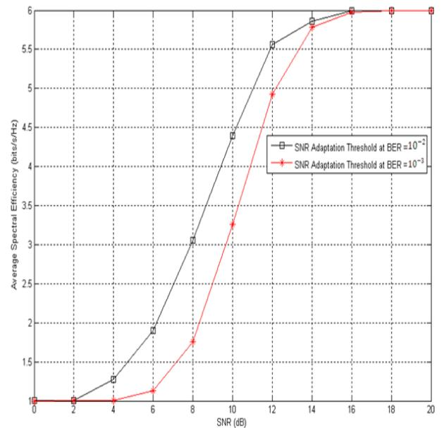
Figure 13. ASE of the proposed cooperative system with combined ACM and BRS, SNR adaptation thresholds at different BER levels ( $BER = 10^{-2}, 10^{-3}$ ),  $N=8$
