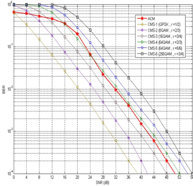
Figure 7. BER performance comparison between direct transmission with different CMSs and with ACM
