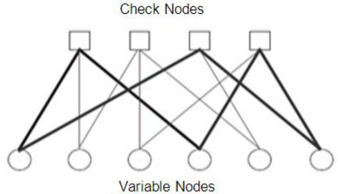
Figure 3. Tanner graph representation of the parity-check matrix in (18), where the bold lines represent 6-cycle
