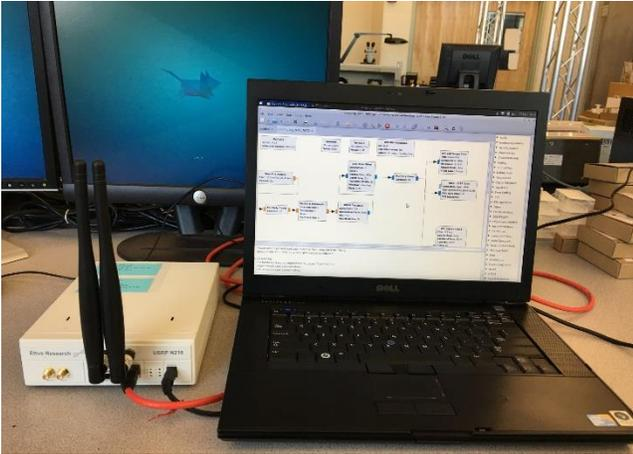
Figure 2: Community radio transmitter using PC, and USRP N210.
