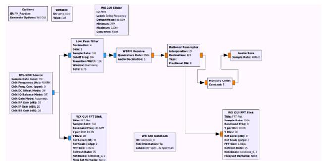
Figure 5: CR receiver flow graph.
