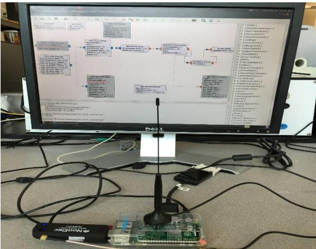
Figure 3: Community radio receiver using Raspberry PI, and RTL-SDR dongle.
