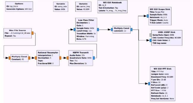
Figure 4: CR transmitter flow graph.
