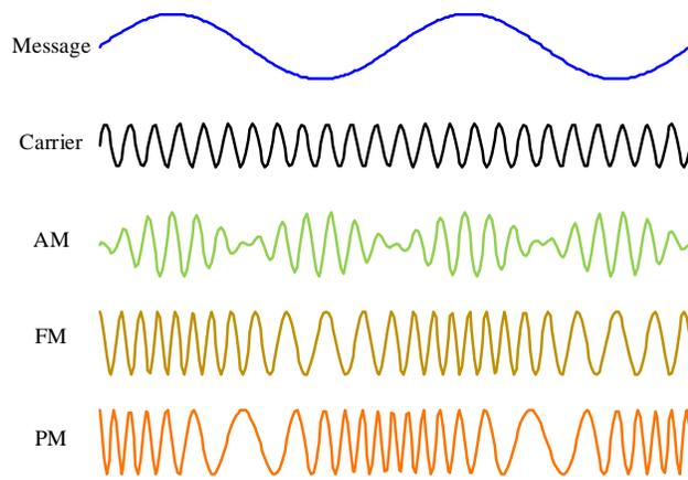
Figure 1: FM and PM modulated signal.
