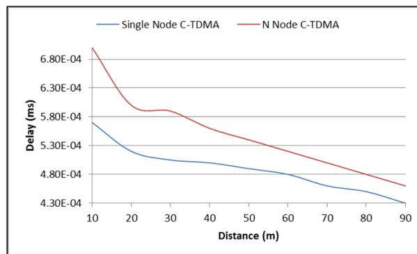
Figure IV-: Delay versus distance
