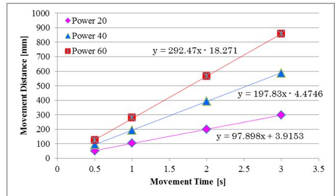
**Figure 4.** Relationship between the time and the distance the robot moved. Functions in the graph represent the approximate linear function.
