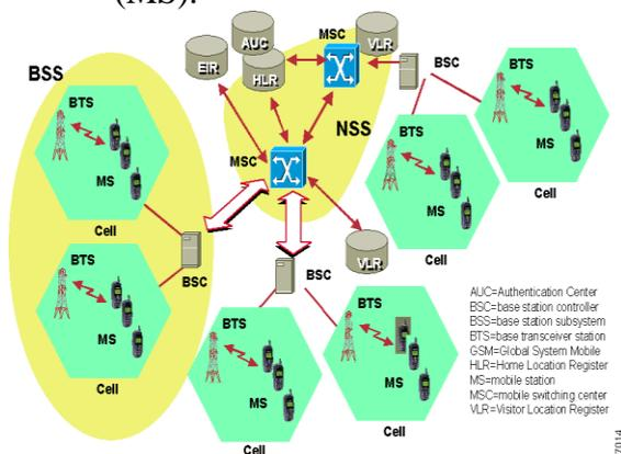
Figure 1: The GSM Networks [5].
