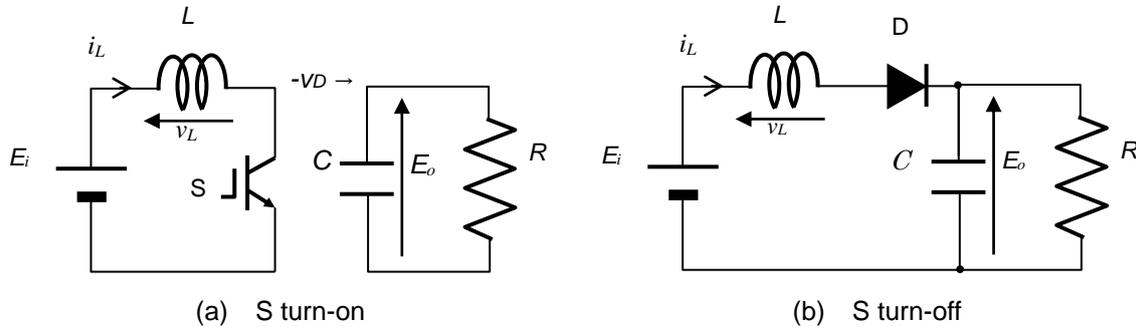
Figure 4. Operating Circuits of Usual Boost Chopper.
