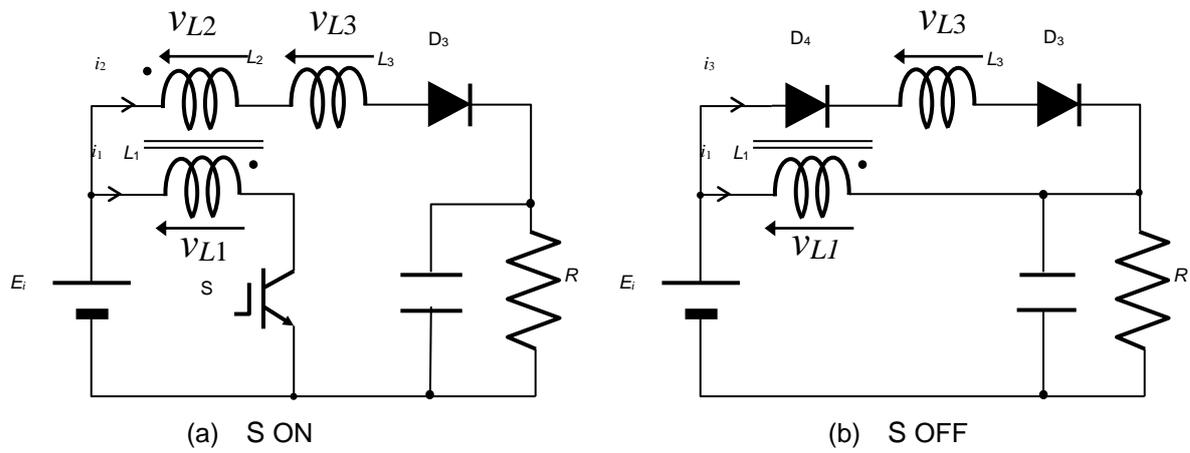
**Figure B. Boost Chopper Having Auxiliary Transformer.**
