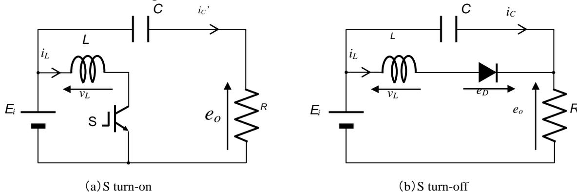
Figure 5. Operation Circuits of Original Boost Chopper.
