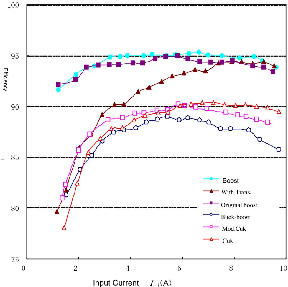
Figure 9. Experimental Results for Various Boost Choppers.
