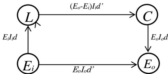
Figure 6. Power Flowchart of Conventional Boost Chopper.
