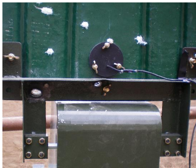
Figure 5: Bullet-Impact Sensor Mechanical Placement
