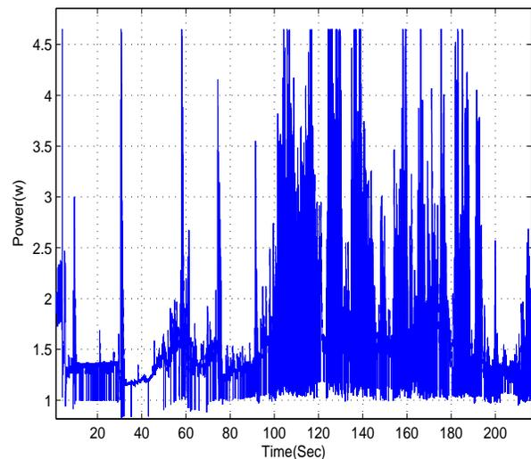
Fig. 12: Emulated power of the DUT during a FTP upload when the device is in a moving car
