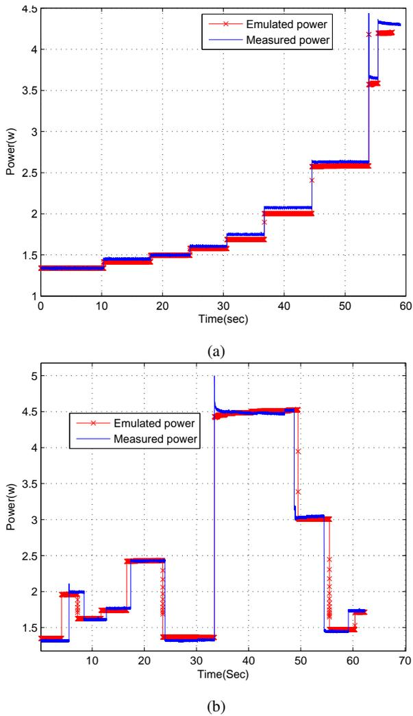
Fig. 11: Power emulation validation: (a) Tx power increasing between  $[-6\ 23]$  dBm and (b) randomly alternating Tx powers
