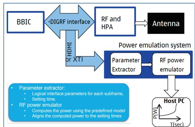
Fig. 1: The RF power emulation system, monitors the stream of the logical commands over the DIGRF interface, extracts the RF subsystem power dependent parameters in the “Parameter extractor” module and computes the emulated power in the “RF power emulator” module.
