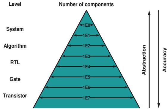
Fig. 2: SOC design levels of abstraction (source [11]) showing that the abstraction decreases, as more knowledge is gained about the SOC. Thus, the power estimation approach after the transistor level presented in this work should be more accurate than the status quo approaches at the system level of abstraction.
