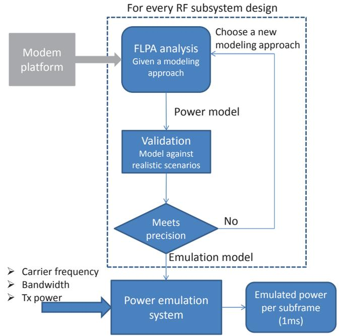
Fig. 10: Emulation flow showing the process through which the emulation model of a RF subsystem is obtained.
