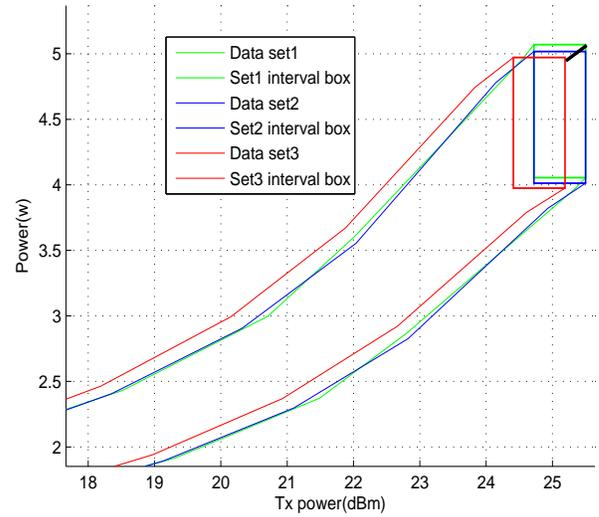
Fig. 7: The buffer zones of three independent measurements used to calculate the Hausdorff distance
