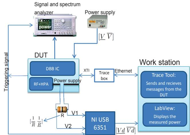
Fig. 5: Power measurement setup used for the measurements in this work. The workstation forces the DUT into a specific mode of operation. During the operation, the DUT power consumption is measured by NI USB and displayed in LabView. The signal analyzer measures the output Tx power at the antenna port
