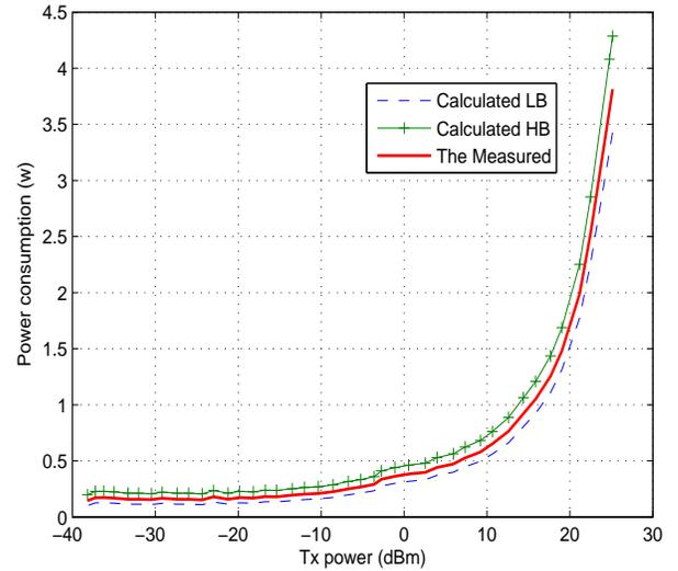
Fig. 8: Measured RF subsystem power consumption operating at 1950 MHz with 10 MHz operational bandwidth and QPSK modulation alongside the calculated lower and upper bounds.
