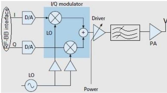
Fig. 4: Direct up conversion transmitter RF subsystem architecture (modified from [28]) of the device used for the experiments in this work. The digital in-phase (I) and quadrature (Q) data from the BB are analog converted, mixed with a RF signal from the local oscillator (LO) and amplified by the PA. The resultant signal is transmitted by the antenna.
