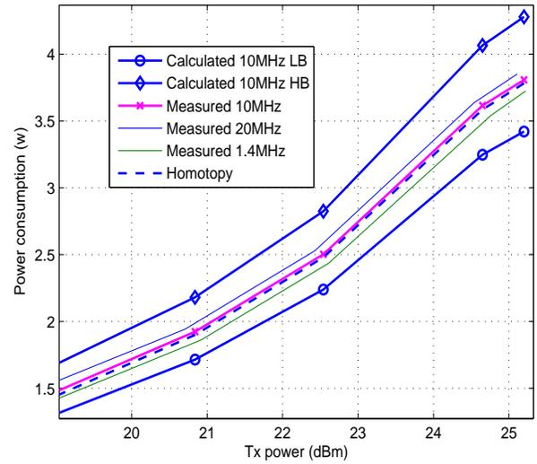
Fig. 6: Homotopical modeling of the RF subsystem power consumption operating at 10 MHz. Only a range of Tx powers is shown for clarity, but the curves are calculated down to -40 dBm.
