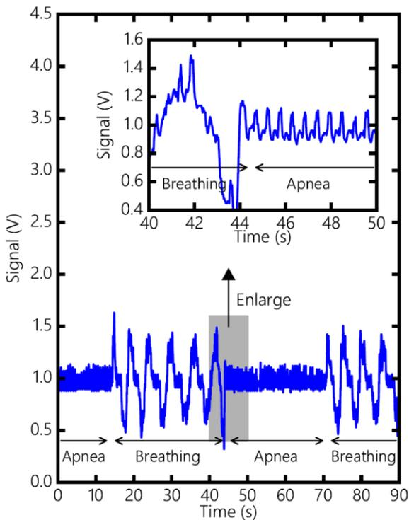
**Figure 5.** The Output signals of the respiration sensor recorded by the data logger. The waveform baseline is at 1.0 V. The respiration status (ventilation or apnea) is clearly distinguishable as large positive and negative peaks appear while the subject is breathing. The inset shows an enlarged waveform between 40 and 50 s. Small peaks are confirmed to be the heartbeat signals of the subject.
