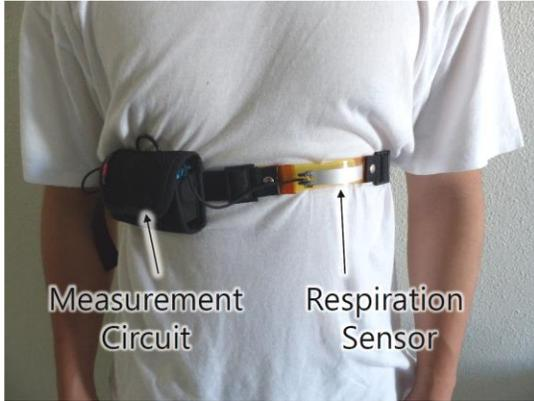
**Figure 4.** The respiration sensor and the measurement circuit worn by a subject (Male, 22 year-old).
