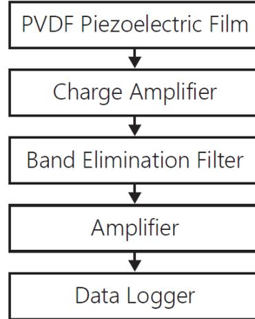
**Figure 3.** Block diagram of the measurement circuit for the respiration sensor.
