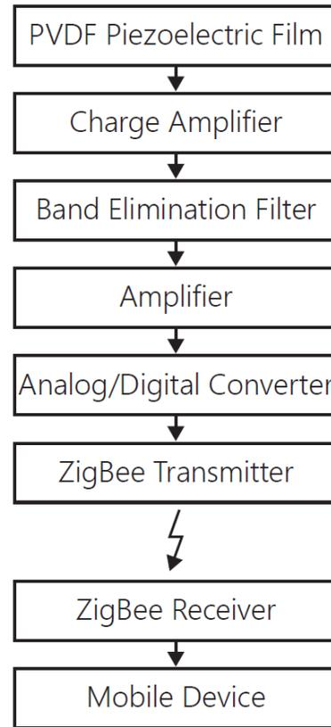
**Figure 7.** Block diagram of wireless monitoring system for the respiration sensor.
