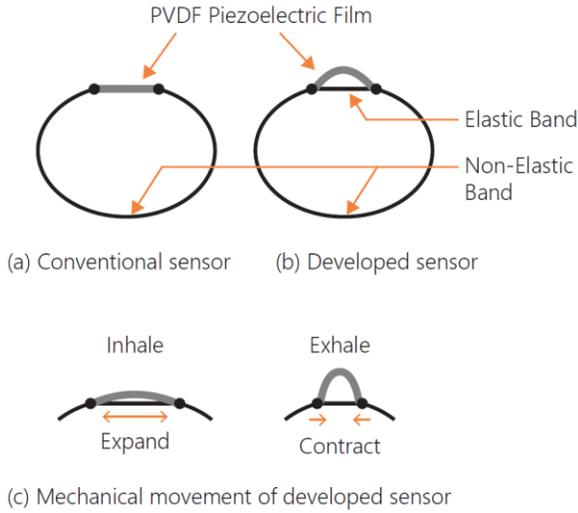
**Figure 2.** (a) Structure of the conventional respiration sensor using piezoelectric film. (b) New structure of the respiration sensor developed in this study. (c) Mechanical movement of the sensor developed following respiration (inhale and exhale) activities.
