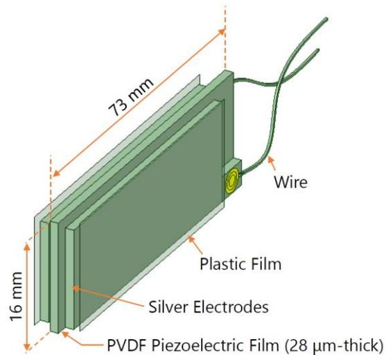
**Figure 1.** Schematic of PVDF piezoelectric film (DT2-028K/L, Tokyo Sensor Co. Ltd.) used for development of the respiration sensor.
