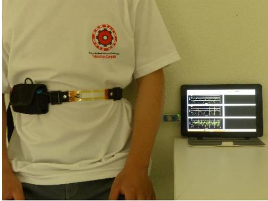
**Figure 8.** The wireless monitoring system for the respiration sensor. The respiration and the heartbeat waveforms are displayed on the tablet computer.
