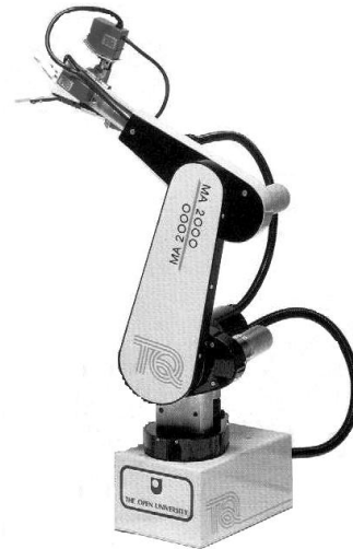
Figure 1. MA2000 robotic manipulator structure.
