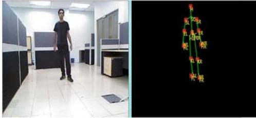
**Figure 4.** 12 Detect joints within the ROI of fall detector
