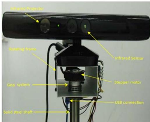
**Figure 9.** Infrared sensor on the custom made stand.
