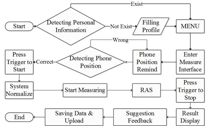
Figure 5. System process flow diagram.
