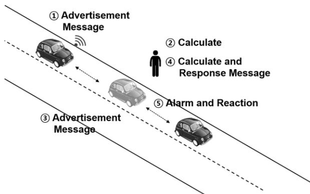
Figure 4. Alarm model of safety distance
