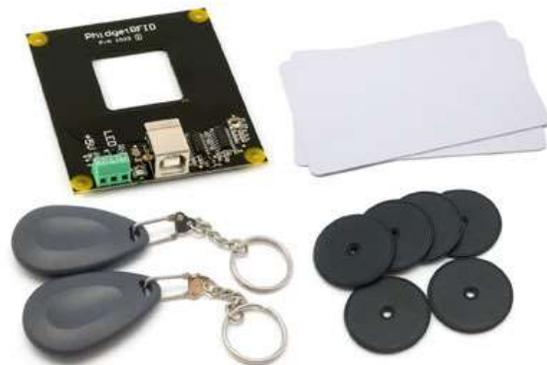
Figure 4 RFID reader and tags
