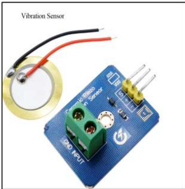
Figure 4: Vibration sensor
