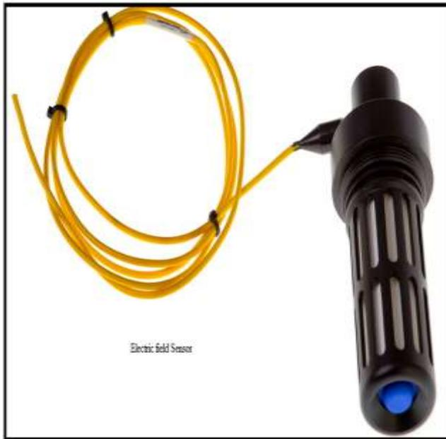
Figure 6: Electric Field Sensor
