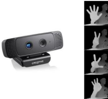
Figure 10: Sens3D (RGB-D Camera)
