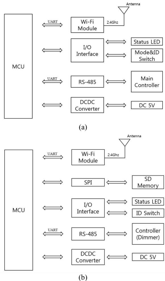
**Figure 3.** A Schematic Diagram of Proposed WDMX: a) is transmitter and b) is receiver.
