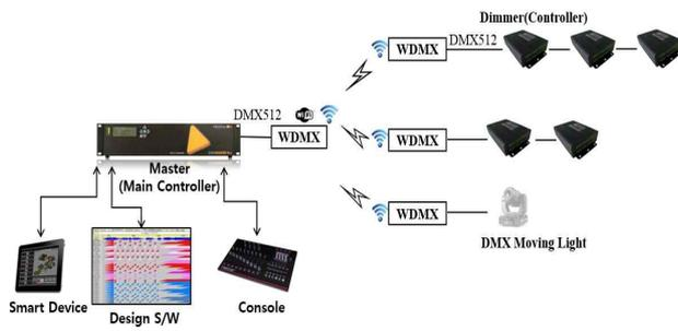
**Figure 2.** A Proposed Wireless Lighting Control System.
