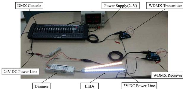
**Figure 5.** A WDMX Test Environments.
