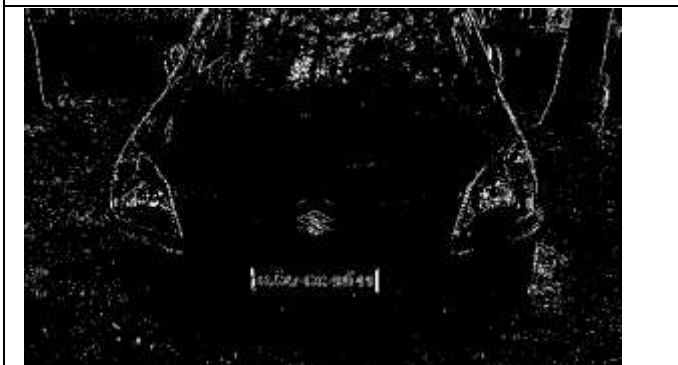
Figure 10(a) Frequency Domain Filtered image with threshold \text{abs}(gf) > 0.2 * \text{abs}(\text{max}(gf(:)))
