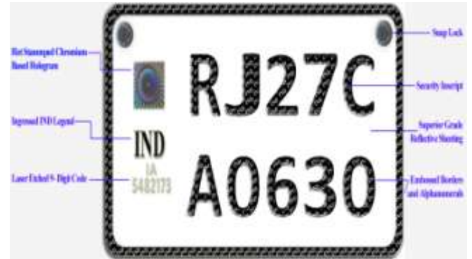
Figure 2. High Security Number Plate with features
