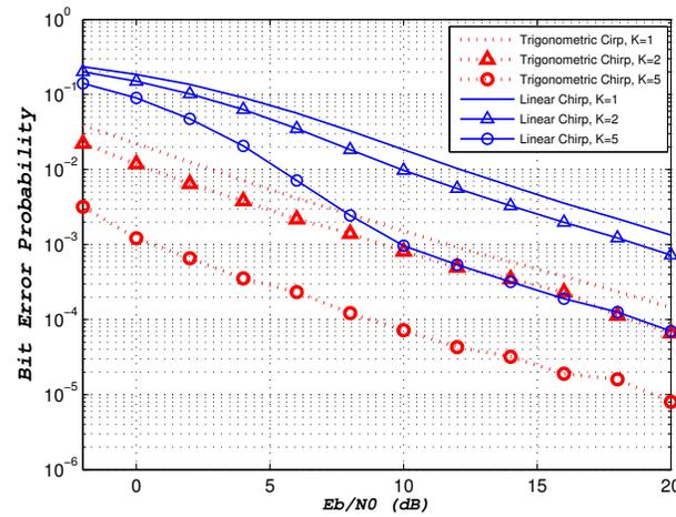
Fig. 7: Linear and Trigonometric chirp Bit Error Rate over Rician Channel,  $BT = 4$ .
