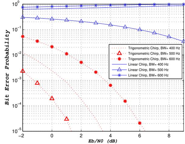
Fig. 3: Linear and Trigonometric chirp BER over AWGN Channel, T = 20 ms.
