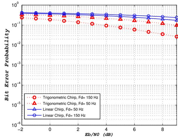
Fig. 6: Linear and Trigonometric chirp Bit Error Rate over Rayleigh fading Channel,  $BT = 4$  and  $f_c = 8kHz$ .
