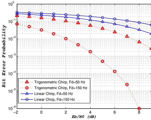
Fig. 4: Linear and Trigonometric chirp Bit Error Rate over Noisy and Doppler Channel,  $BT = 4$  and  $f_c = 8kHz$ .
