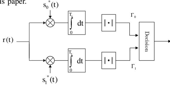
Fig. 1: Block Diagram of Optimum Non-Coherent Detector.
