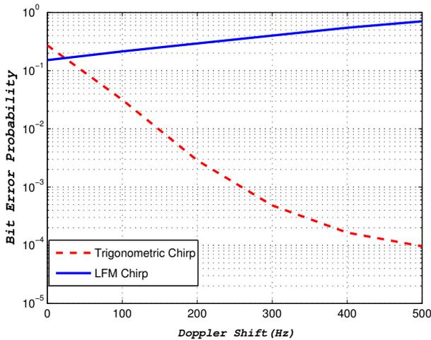
Fig. 5: Linear and Trigonometric chirp Bit Error Rate vs. Doppler Shift,  $BT = 4$ ,  $SNR = 2$  dB and  $f_c = 8kHz$ .
