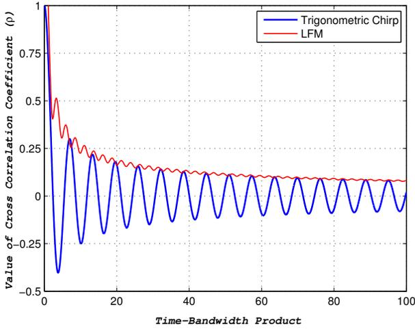
Fig. 2: Correlation Coefficient for LFM and Trigonometric Chirp.
