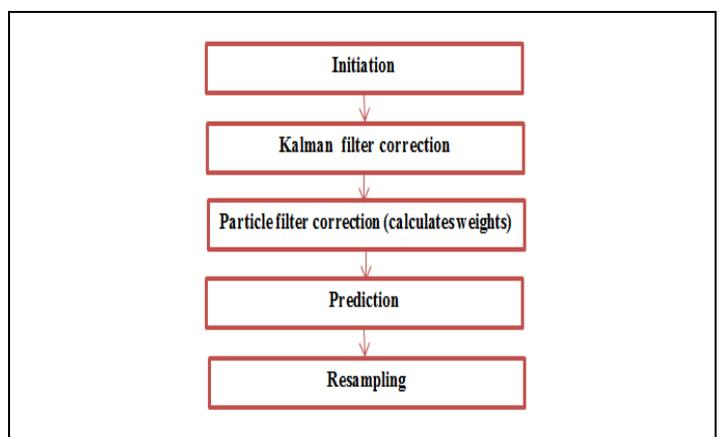
Fig. 3. Kalman-Particle Kernel Filter diagram.
