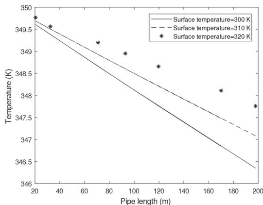
**Fig. 6.** Effect of surface temperature on water outlet temperature.
