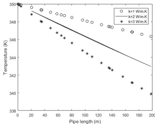
**Fig. 3.** Effect of soil thermal conductivity on water outlet temperature.
