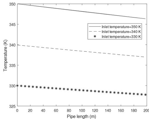
**Fig. 5.** Effect of fluid inlet temperature on water outlet temperature.
