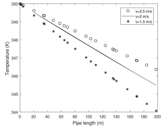
**Fig. 4.** Effect of fluid velocity on water outlet temperature.
