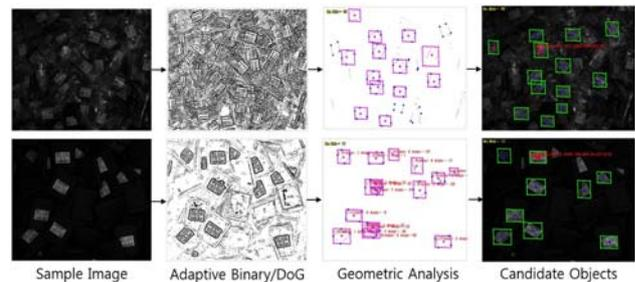
Figure 3. Candidate object detection using simple cue in low resolution image
