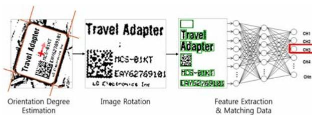
**Figure 6.** The training process for pose estimation using neural network
