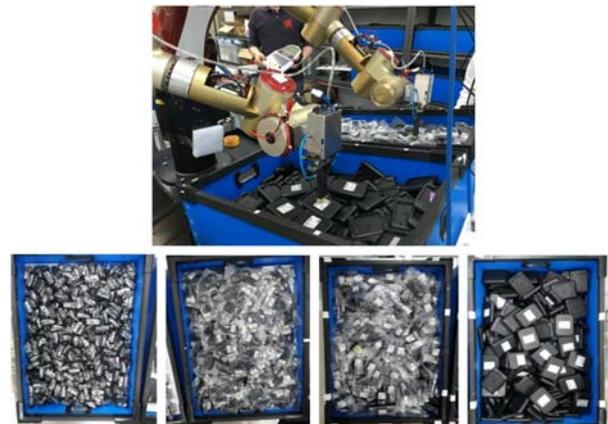
**Figure 7.** Bin picking using dual arm robot
