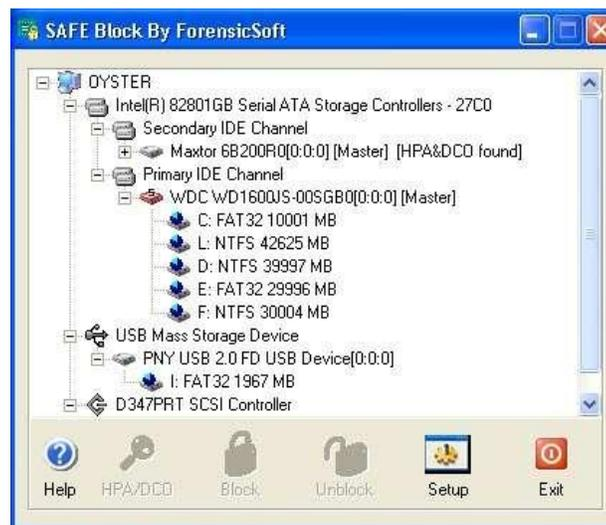
Figure 6. Software Write Blocker: SAFE Block Win 7 64 bit
