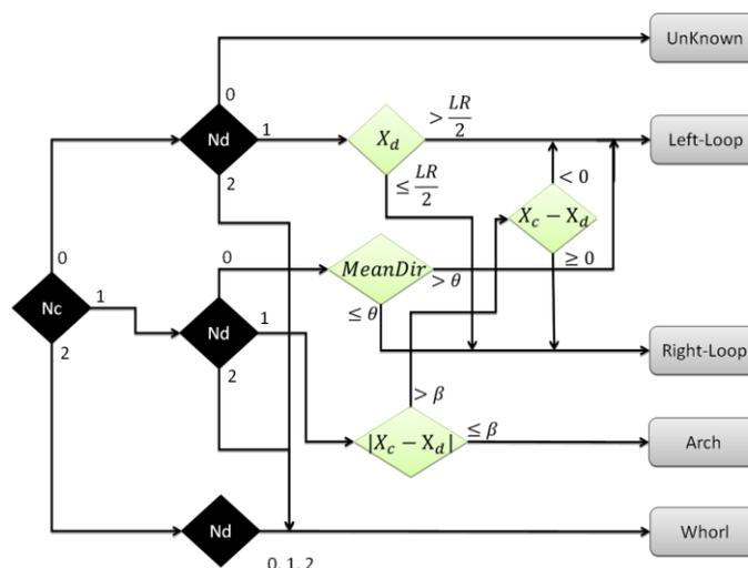
**Figure 2.** Proposed rules for fingerprint classification based on singular points information
