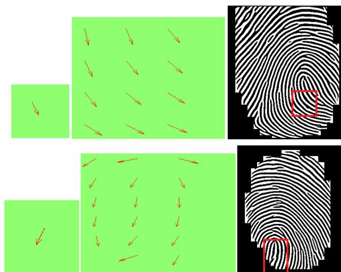
**Figure 6.** First row: Right loop class - Second row: Left loop class (a) Neighborhood area (b) Blocks direction in the area (c) Average direction of blocks (MeanDir)
