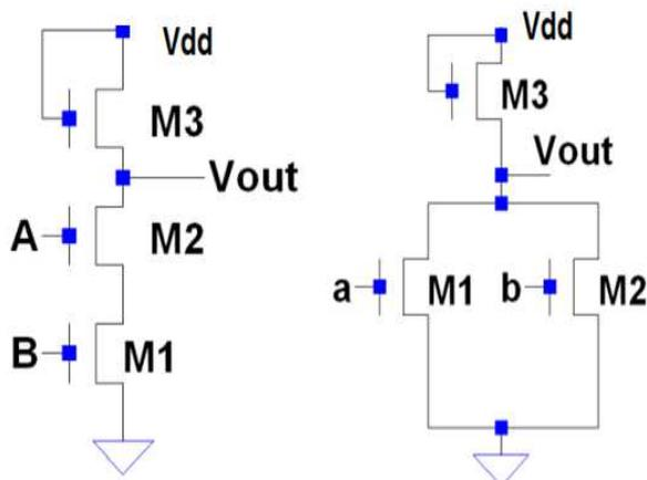
**Figure 4.** a-Si NAND gate(a) and a-Si NOR (b) gate configurations.
