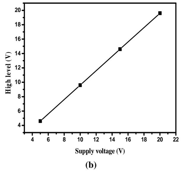
**Figure 6.** High (a) and Low (b) levels vs supply voltage for a-Si NAND gate.
