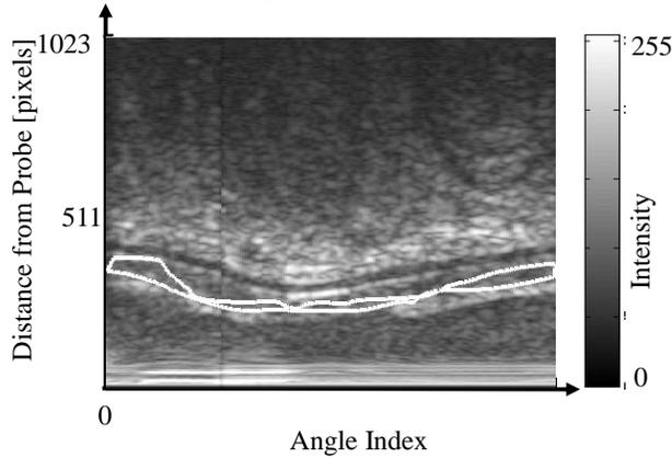
**Figure 8.** Initial contour of the new modified level set.
