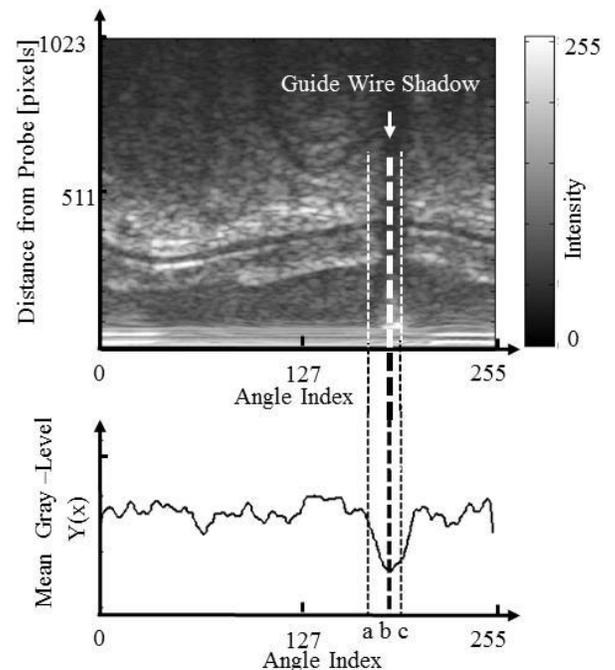
Figure 4. Guide wire shadow detection.
