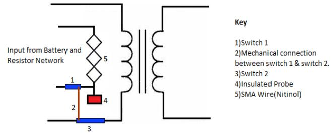
**Figure 5 :** Experimental Setup for using a SMA as a relay.
