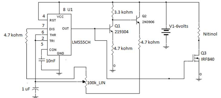
Figure 7 :555 IC timer circuit used for Pulse Width Modulation.
