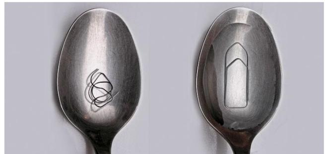
**Figure 1:** This image shows the transformation of the material from deformed martensitic stage to parent state when immersed in warm water. After the clip is removed from water, its dimensions remain same even though internally it undergoes a transformation from parent to twinned martensite state.
