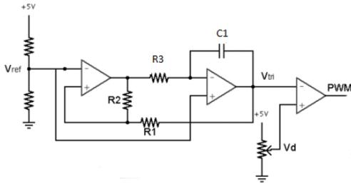
**Figure 9 :** This circuit gives an alternate method to produce pulse width modulated current for the nitinol wire.
