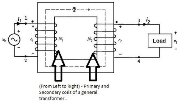
**Figure 4 :** A general transformer that is present within every consumer electronic device for stepping down the voltage.
