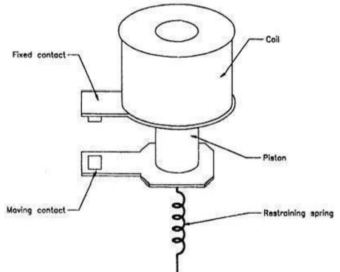
Figure 3 : A general relay mechanism. The piston shown moves down to compress the spring due to the magnetic force exerted by the coil, when an electric current flows through it. The spring sends it back to its original state when the circuit needs to be changed.
