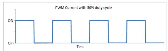
Figure 8 :Pulse width modulated wave generated by 555 with duty cycle of 50% to stimulate the wire.
