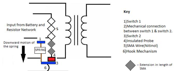
**Figure 6 :** Representation of the experimental setup to restore SMA to original position.
