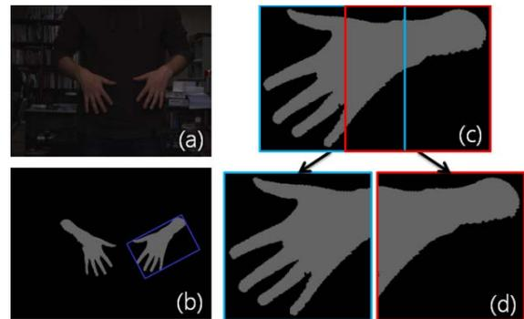
**Figure 3.** Hand-arm region detection and separation when a user wore a long-sleeve shirt and rolled up his/her sleeves. (a) Input scene, (b) hand-arm regions, (c) minimum bounding rectangle surrounding a hand-arm region, (d) hand-arm region separation.
