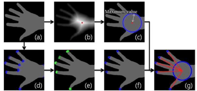
**Figure 6.** Hand shape recognition. (a) Input hand region, (b) distance transformed hand region, (c) palm detection result, (d) fingertip candidates, (e) refined fingertip candidates, (f) fingertip detection result, (g) hand shape recognition.
