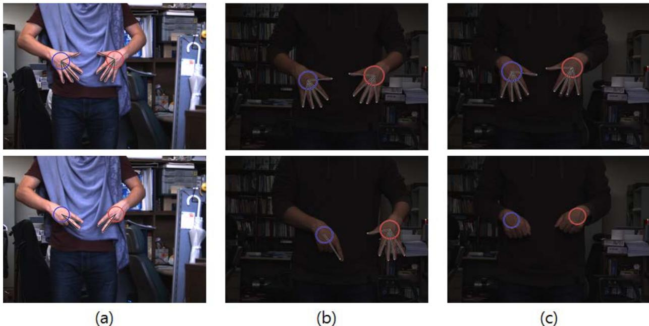
**Figure 7.** Various results of the proposed method. (a) Results when a user wore a short-sleeve shirt with high illumination, (b) results when a user wore long-sleeve shirt and rolled up one's sleeves with low illumination, (c) results when a user wore a long-sleeve shirt with low illumination.
