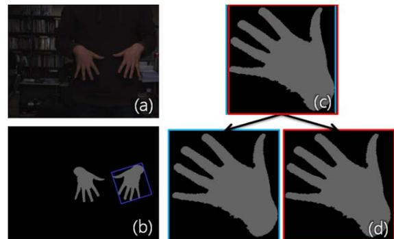
**Figure 4.** Hand-arm region detection and separation when a user wore a long-sleeve shirt. (a) Input scene, (b) hand-arm regions, (c) minimum bounding rectangle surrounding a hand-arm region, (d) hand-arm region separation.
