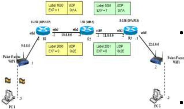
**Figure 8.** L-LSP mechanism with QoS
