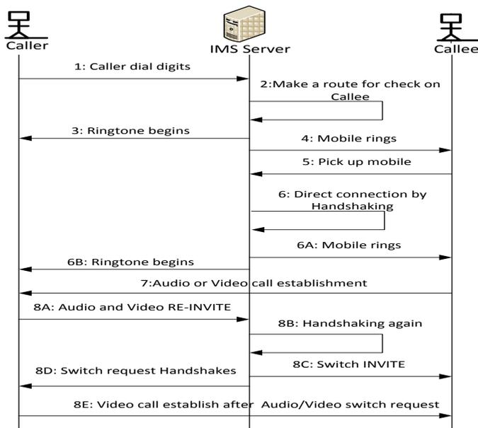
Figure 3. Flow Diagram Of Call Switching Between Caller and Callee Through IMS Flow At Different Stages
