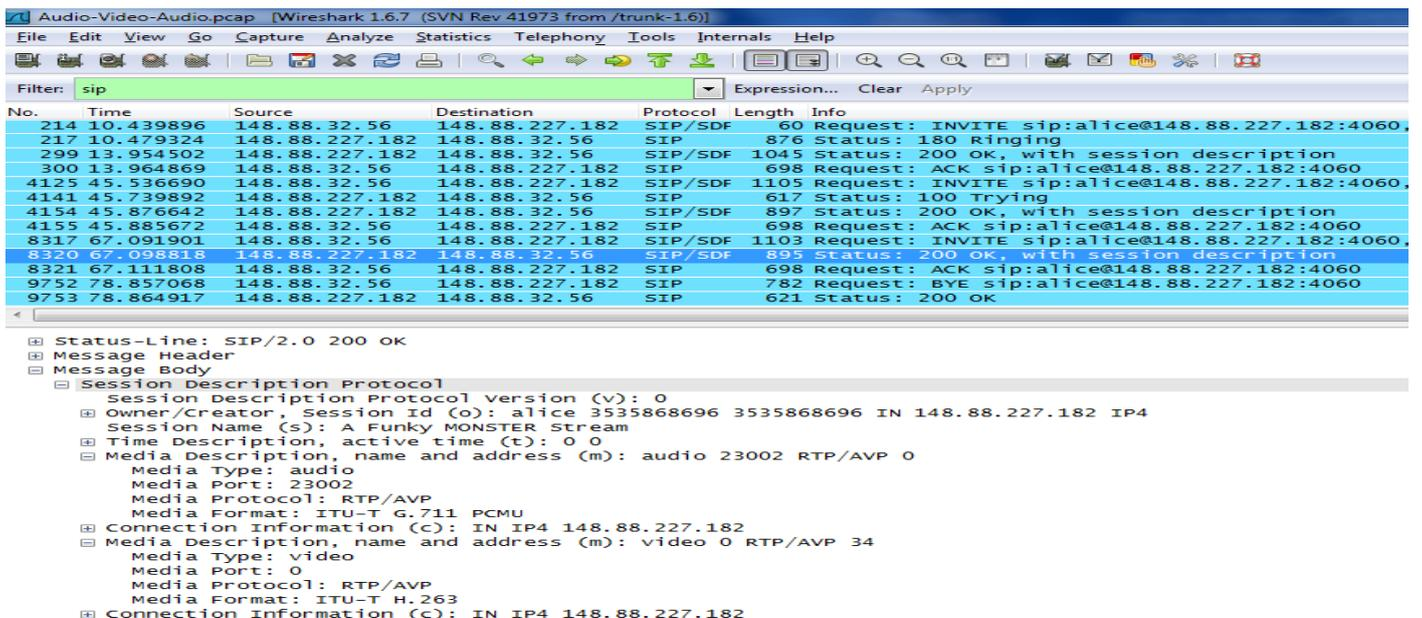
Figure 9. Data Of Video Codec Block, During Switching From Video To Voice Call
