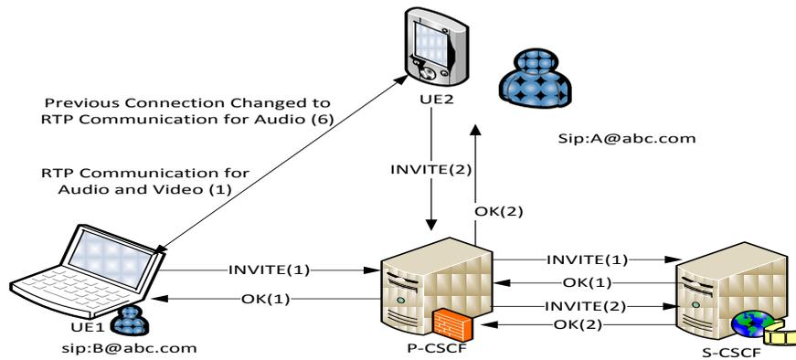
Figure 5. Flow Of Invite Request For Audio/Video Call Establishment
