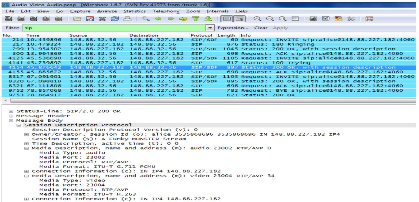
Figure 8. Data Of Voice and Video Codec Sharing During Voice To Video Call Switching
