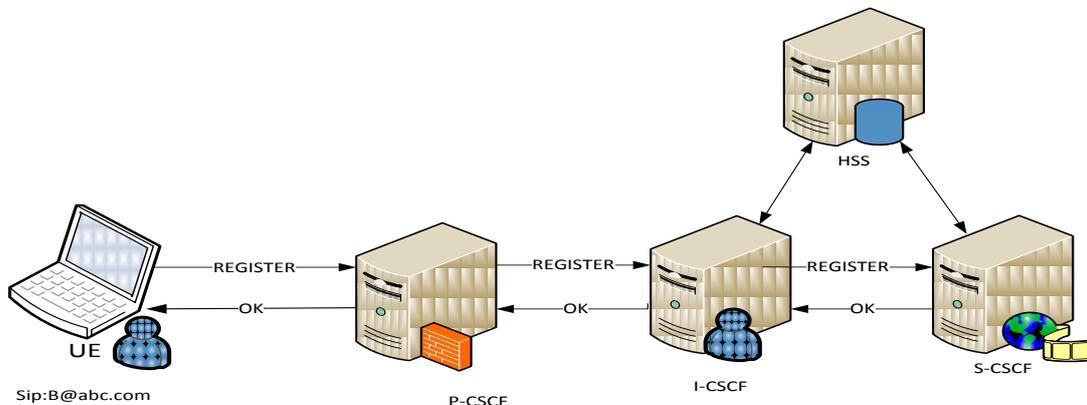
Figure 4. Registration From IMS Client To IMS Network
