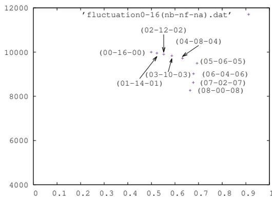
Fig. 10. The fundamental diagram between nb-nf and nb-f by adding the fluctuation gradually, where x and y axes are car density and the number of traffic flow, respectively.
