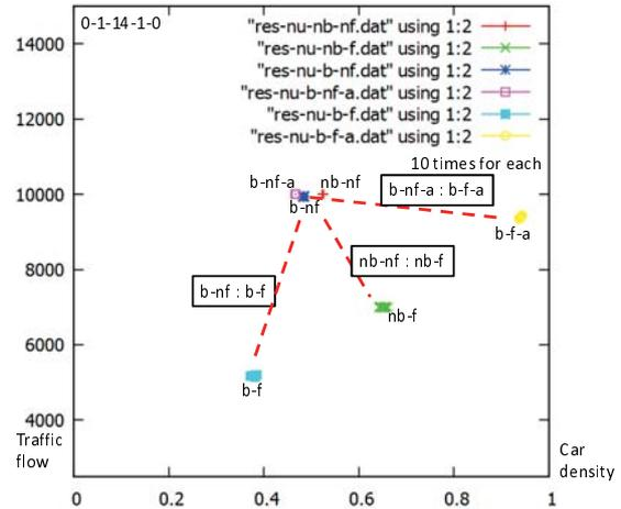
Fig. 8. Traffic flow versus car density relationships among car driving types: the probabilities for the speed 0, 1, 2, 3 and 4 correspond to  $0, \frac{1}{16}, \frac{14}{16}, \frac{1}{16}$  and 0, respectively.
