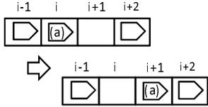
Fig. 5. Shortening one cell too close a car in front in minimum boundary effects.
