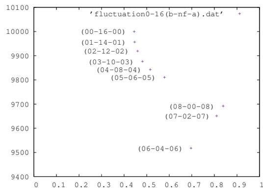
Fig. 9. The fundamental diagram between b-nf-a and b-f-a by adding the fluctuation gradually, where x and y axes are car density and the number of traffic flow, respectively.
