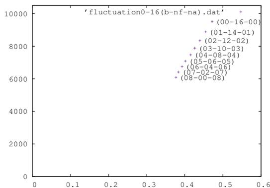
Fig. 11. The fundamental diagram between b-nf and b-f by adding the fluctuation gradually, where x and y axes are car density and the number of traffic flow, respectively.
