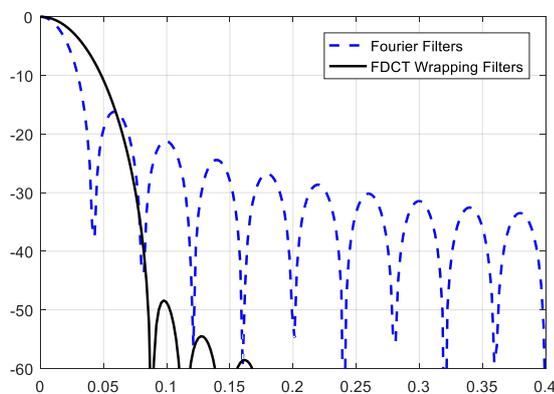
**Figure 7.** Frequency response of Fourier and FDCT wrapping for OFDM transmission.
