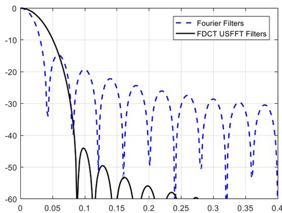
**Figure 6.** The frequency response of Fourier and FDCT USFFT for OFDM transmission.
