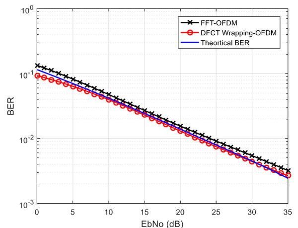
**Figure 9.** BER performance of OFDM system based on FDCT via wrapping.
