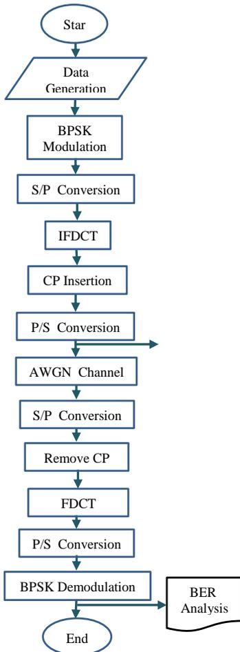
**Figure 5.** Simulation procedures of the OFDM system based on FDCT.
