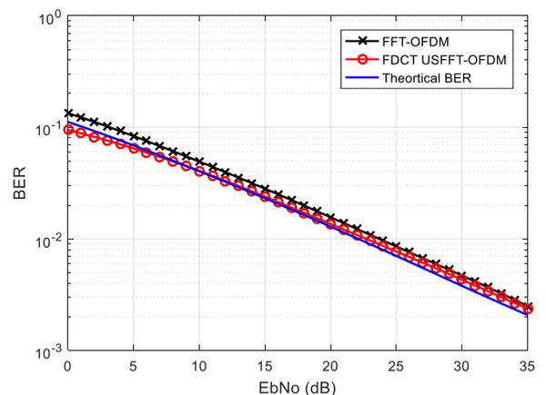
**Figure 8.** BER performance of OFDM system based on FDCT via USFFT.
