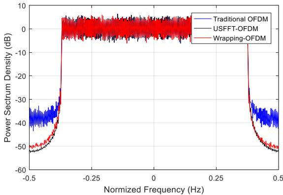
**Figure 10.** PSD for the proposed and conventional OFDM systems.
