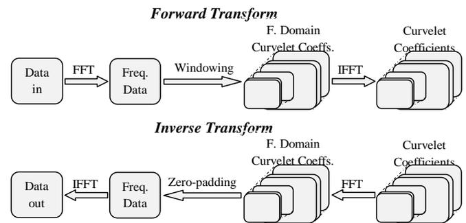
**Figure 3.** Data flow for the Forward and inverse wrapping FDCT.
