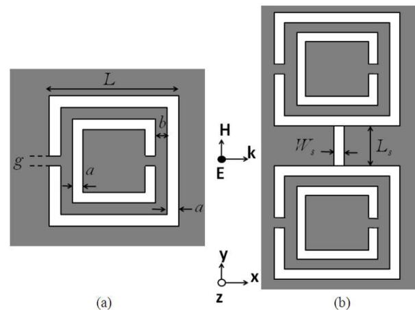
**Fig. 2** (a) CSRR unit cell, and (b) the proposed slotted-CSRR inclusion. Note that gray area represents metallization.
