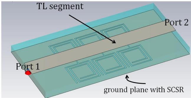
**Fig. 11** 3D view of the bandstop filter with slotted-complementary spiral resonators etched out from metallic ground plane. Note that TL segment is matched to  $50\Omega$ .
