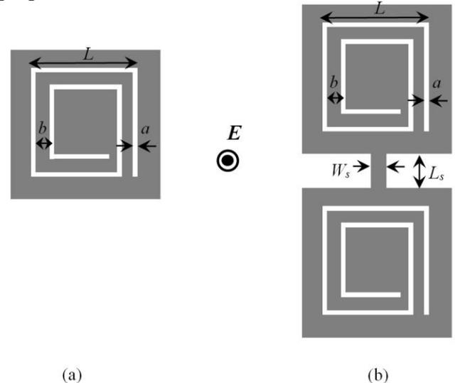
**Fig. 7** (a) Complementary spiral resonator (CSR) unit cell with its relevant dimensions, and (b) the proposed slotted-CSR unit cell. Note that gray area represents metallization.
