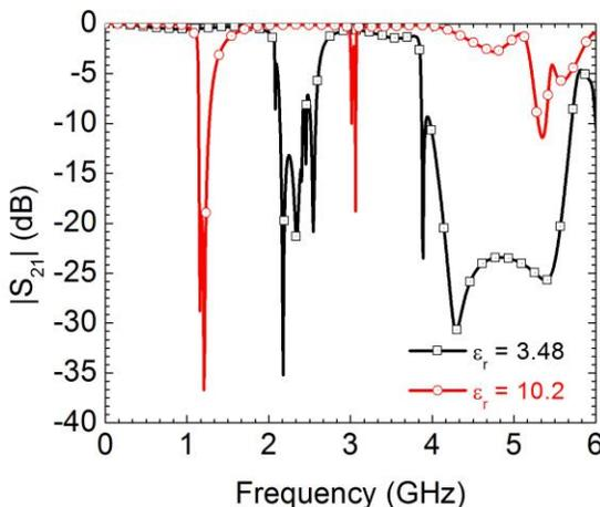
**Fig. 12** Simulated transmission coefficient,  $S_{21}$ , for the filter with slotted-CSRs (S-CSRs).
