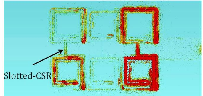
**Fig. 13** Snapshot for simulated surface current distribution along the vicinity of the metallic ground plane of the bandstop filter with Slotted-CSRs at resonant frequency of  $2.1\text{ GHz}$ .
