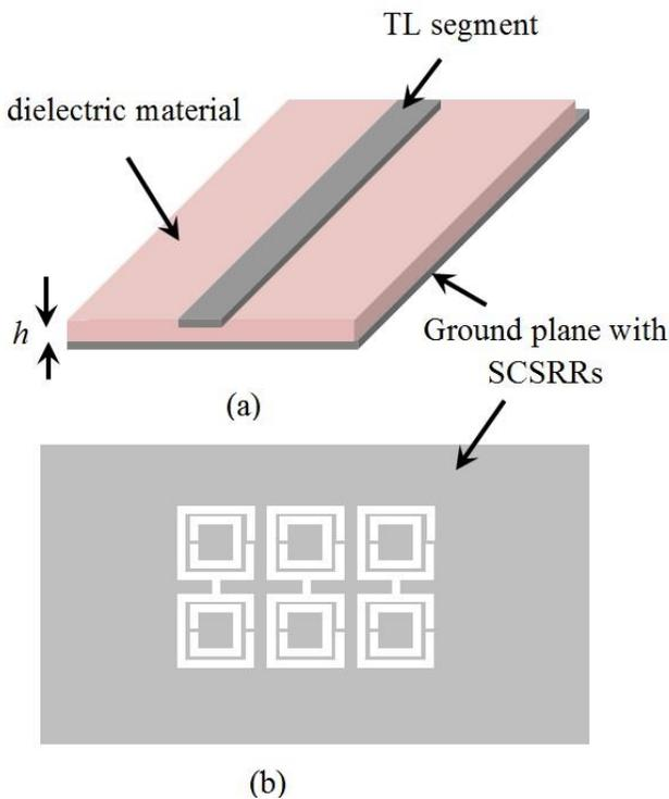
**Fig. 3** (a) 3D view of the bandstop filter with SCSRRs etched from ground plane; (b) bottom view of the bandstop filter with slotted-CSRRs etched from the ground plane.
