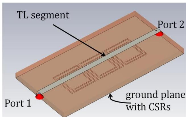
**Fig. 8** 3D view of the bandstop filter with complementary spiral resonators etched out from metallic ground plane. Note that TL segment is matched to  $50\Omega$ .
