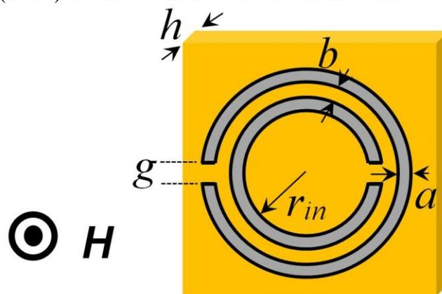
Fig. 1 A split-ring resonator (SRR) particle with its relevant dimensions. Note that gray area represents metallization.
