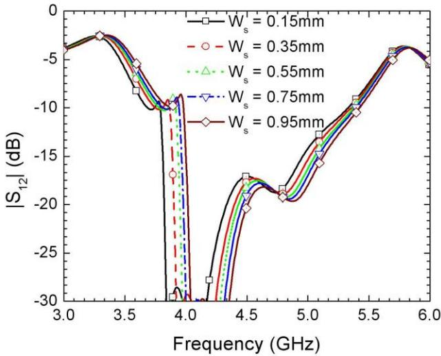
**Fig. 5** A parametric study illustrates the effect of the S-CSRR slot width,  $W_s$ , on the rejection band of the filter.
