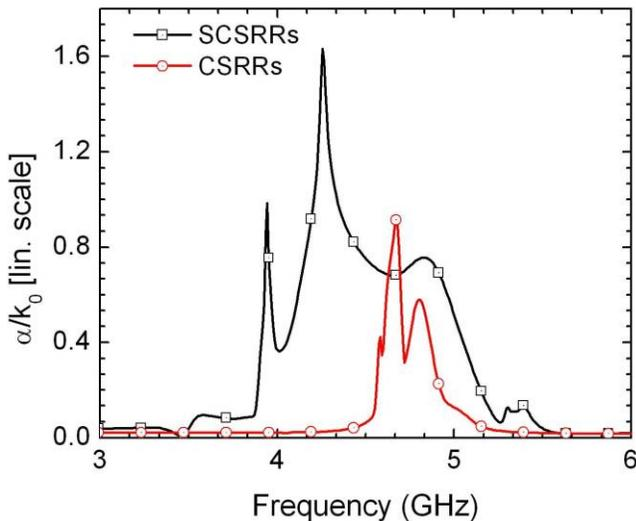
**Fig. 6** Attenuation coefficient for the proposed filter with S-CSRRs and compared with CSRRs filter (without the slot).
