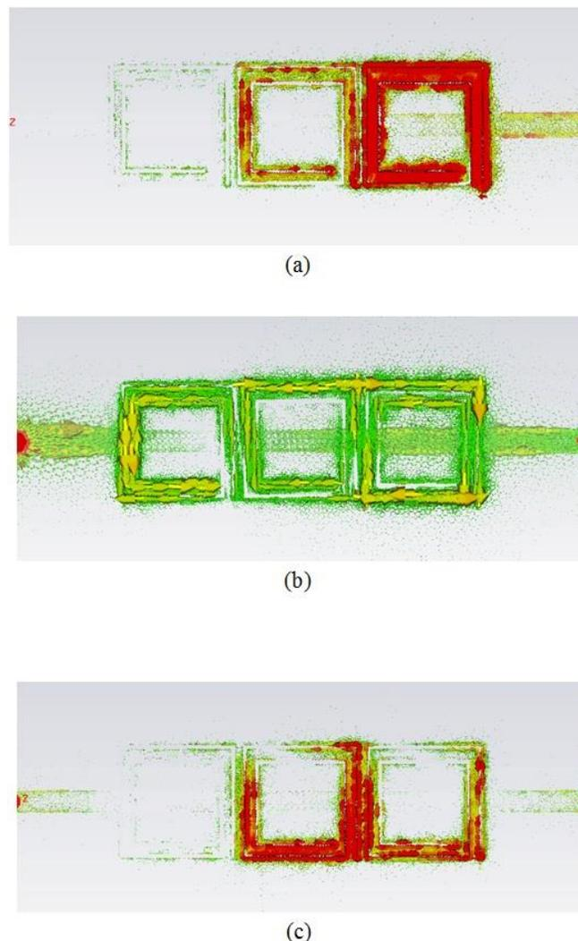
**Fig. 10** Snapshots for simulated surface current distribution along the vicinity of the metallic ground plane of the bandstop filter with CSRs at various frequencies: (a) 1.2 GHz, (b) 2.5 GHz, and (c) 3.0 GHz. Note that no slits are presented for the CSRs.
