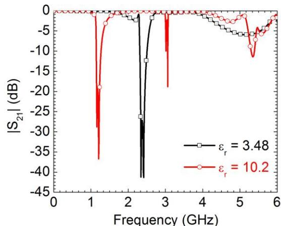
**Fig. 9** Simulated transmission coefficient,  $S_{21}$ , for the filter with CSRs. Note that no slits are presented for the CSRs.
