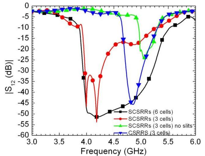
**Fig. 4** Simulated transmission coefficient,  $S_{21}$ , for the bandstop filter with the proposed slotted-CSRRs, and compared to a bandstop filter with classical CSRR inclusions.
