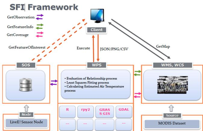
Fig. 1. SFI framework in GEO Grid Architecture GEO GRID Architecture
