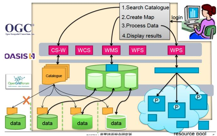
Figure 1: GEO GRID Architecture
