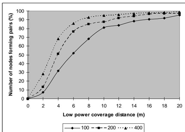
Figure 1 Percentage of nodes forming pairs vs. low power coverage distance (m) for 100, 200, and 400 random nodes in a 100m x 100m field
