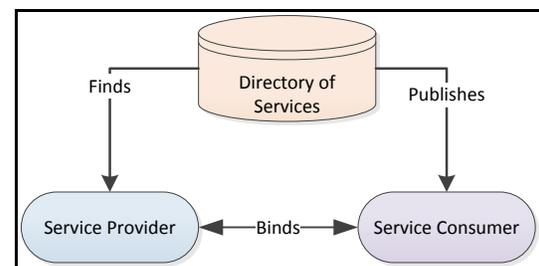
Diagram 1: Concept of Service Oriented Architecture
